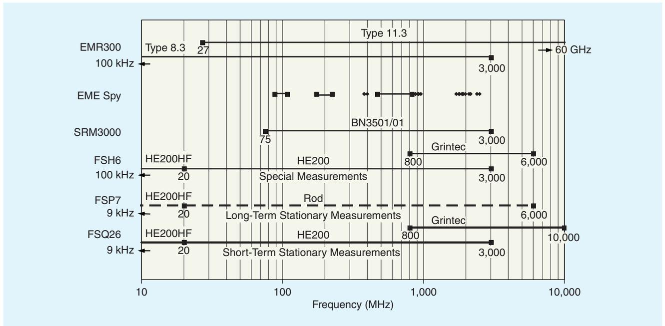
**Table 1: Measurement equipment used: on the left side, the analyzing equipment is indicated. The horizontal lines show the frequency range with the respective sensor indicated above. The style of the lines indicates the type of measurements. 1. bold lines: short term stationary measurements 2. dashed lines: long term stationary measurements. 3. fine lines: special measurements.**
