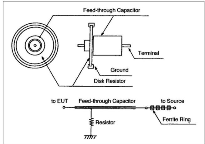
Figure 4. Configuration and circuit diagram of VHF/UHF LISN.
