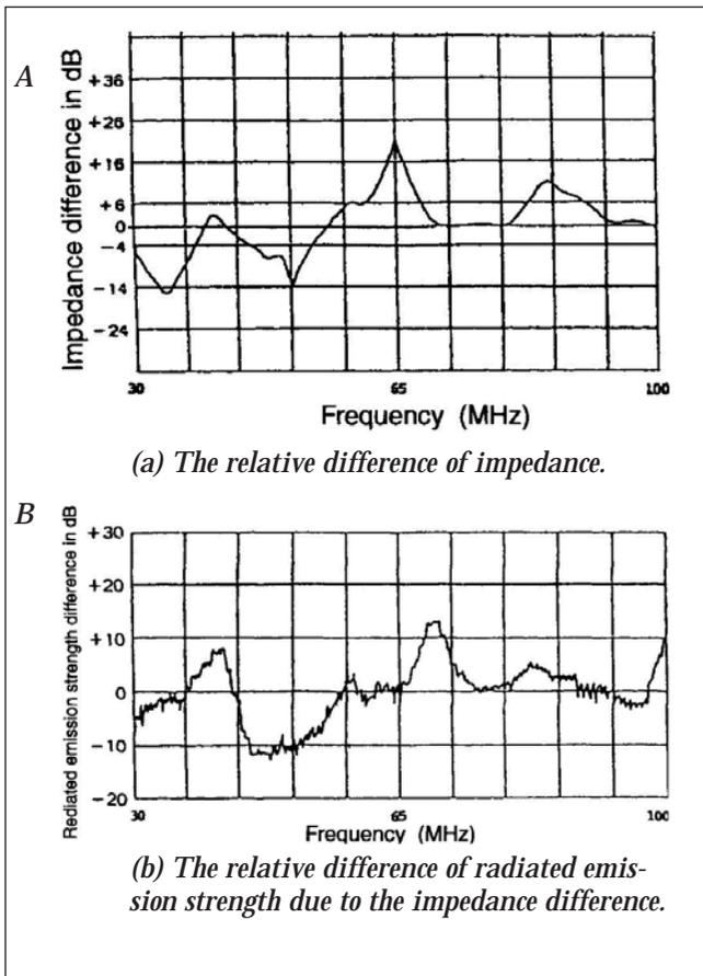
Figure 3. The radiated emission strength difference corresponding to the impedance difference.
