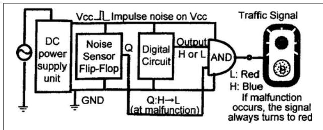
Figure 11. Application to fail-safe control of traffic signal.
