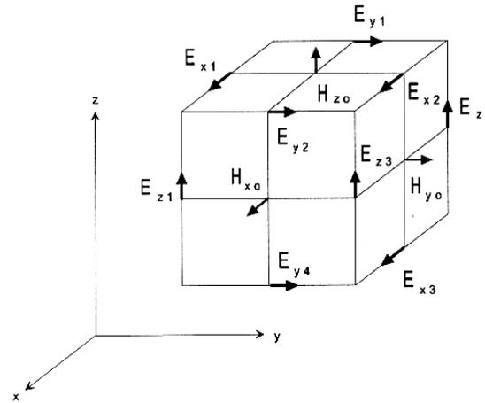
Figure 2: Basic Element of the FDTD Space Lattice
