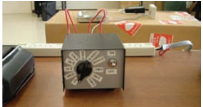
Fig. 2. Measurement setting (a variable resistance box, front, and an antenna, the white box in back).
