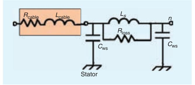
Fig. 11. A high frequency model of a motor with a short cable.
