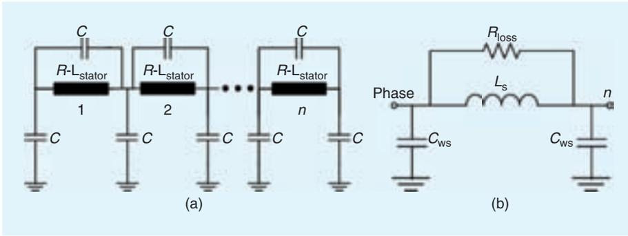
Fig. 6. (a) a distributed model of an electric motor at high frequency (b) a simple model of an electric motor.
