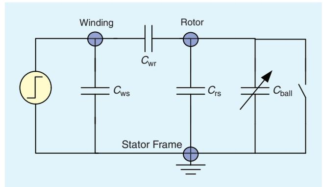
Fig. 5. A high frequency model of an induction motor.
