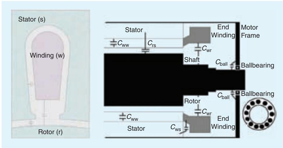
Fig. 2. A view of stator slot and capacitive coupling in an induction motor.
