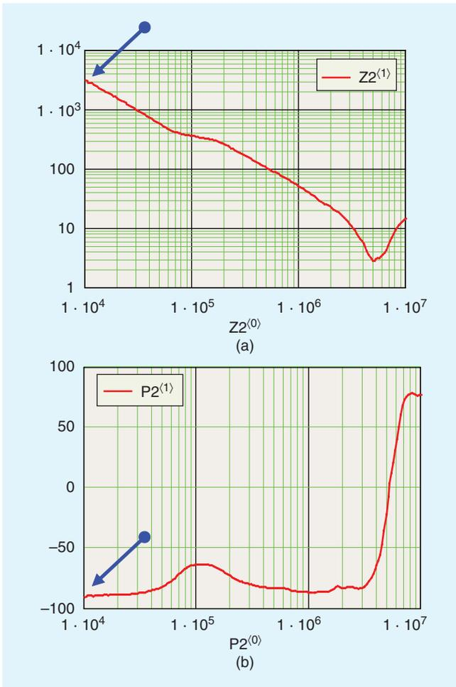
Fig. 8. Measurement results (a) magnitude and (b) phase values between the phases and the stator of a 5.5 KW motor.
