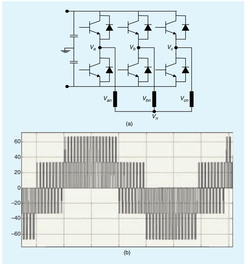
Fig. 4. (a) three phase voltage source inverter (b) PWM voltage.
