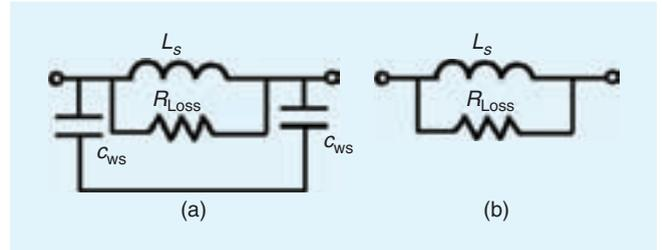
Fig. 9. Circuit diagram for measurement between phases and star point (a) a model of motor (b) simplified model for low frequency range.
