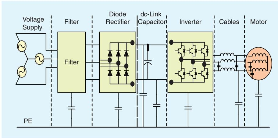
Fig. 1. A power electronic motor drive system with capacitive couplings.
