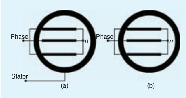
Fig. 7. Two different connections to measure the impedance between (a) the phases and the stator (b) the phases and the star point.
