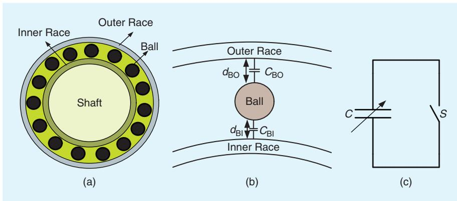
Fig. 3. (a) general structure of a ball bearing (b) a view of ball, outer and inner races and capacitive couplings (c) simple model of a ball bearing.
