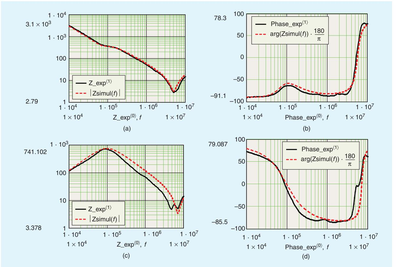
Fig. 12. Experimental and simulation results of a 5.5 kW motor; (a) magnitude (b) phase values between phases-stator (c) magnitude (d) phase values between phases-star point.
