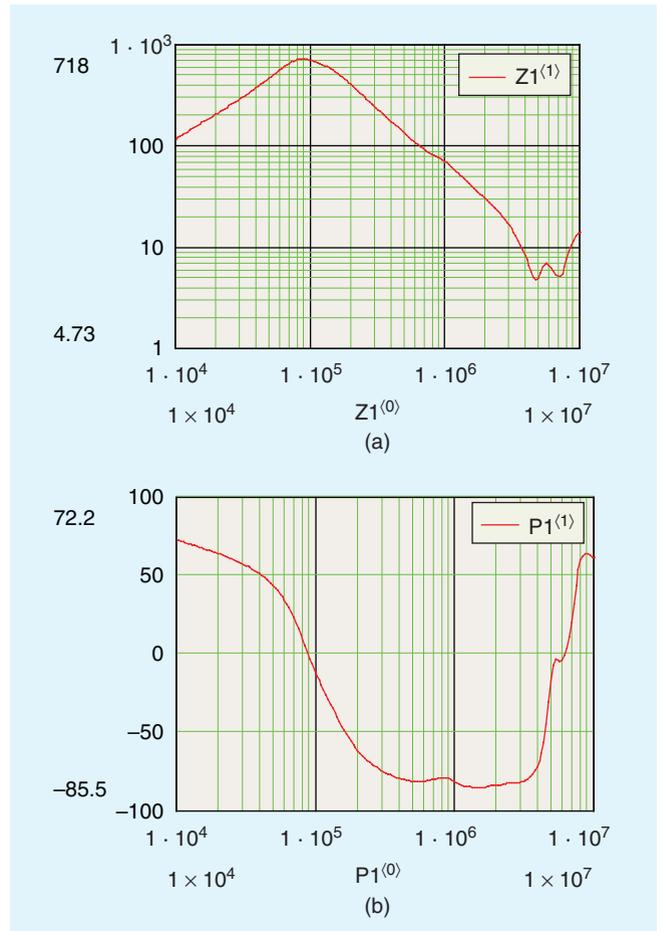
Fig. 10. Measurement results (a) magnitude and (b) phase values between the phases-star point of a 5.5 KW motor.
