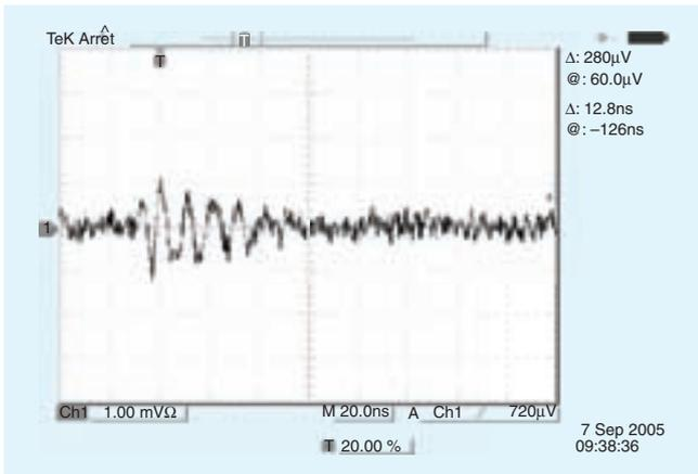
Fig. 8. Pulse measurements. Parasitic signal picked-up by the set-up, without field sensor.
