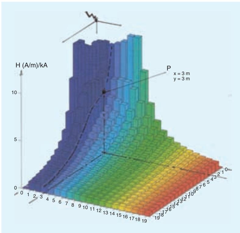
Fig. 4. Example of field distribution in a corner zone, for height  $z = 1.50 \text{ m}$ . H-field values are normalized in (A/m)/kA.
