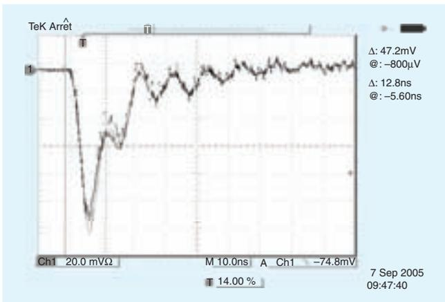
Fig. 9. Pulsed field. Sensor 7.5 cm inside. Only one grid. Scale : Ch.1 : 20 mV = 100 mA/m. The overshoot after the first peak is deemed to be the reflected pulse bounced-back after its two-way trip.
