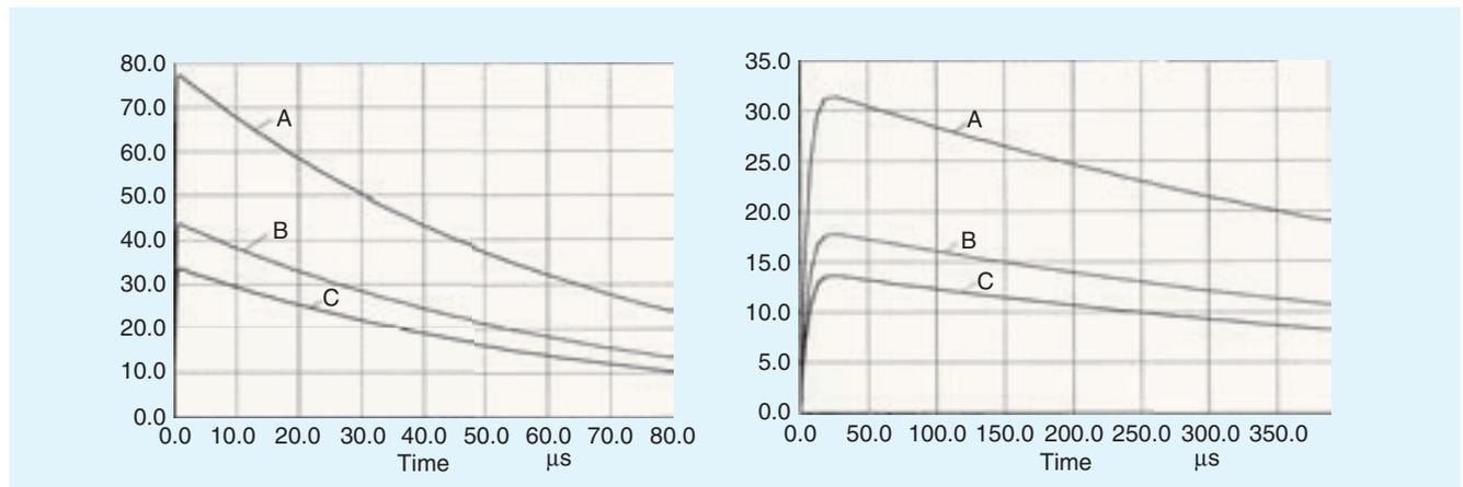
Fig. 5. Structural Voltages in kV, for waveforms #1, slow, 200 kA (top) and #2, fast 50 kA (bottom). Curve A: absolute value of grid voltage of building roof belt vs. remote ground reference. Curve B: absolute value of floor slab voltage vs. remote ground ref. Curve C:  $\Delta V$  (A-B), ceiling-to-floor voltage gradient.
