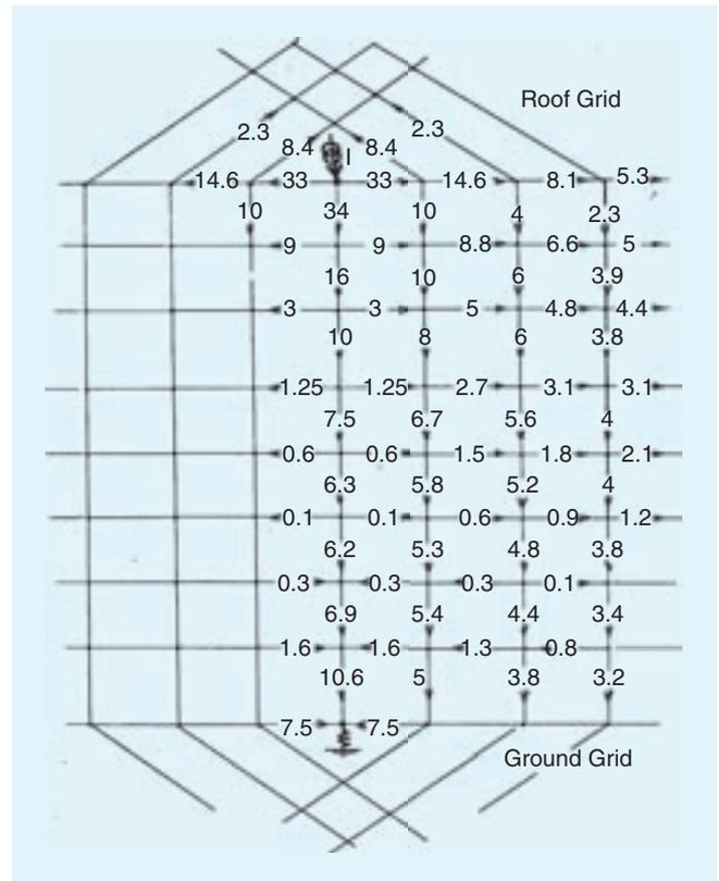
Fig. 3. Example (partial) of currents distribution in grid cells, seen from the inside, for injection at top of a corner zone. The 3-D configuration has been transformed in a 2-D schematic. Currents shown in % of total  $I$  injected. Notice the direction reversal of horizontal currents, from top to bottom.
