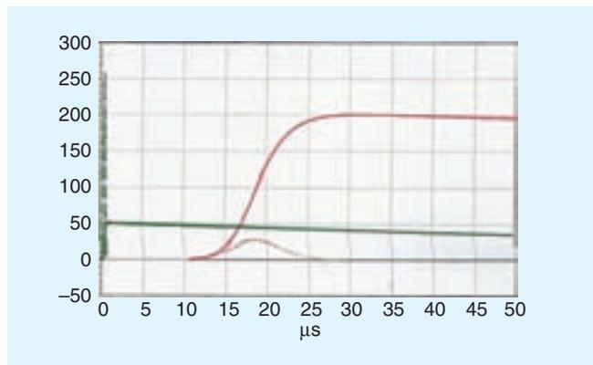
Fig. 1. Lightning Current Waveforms #1 and 2, with respective time derivatives (dotted lines, kA/ $\mu$ s) per IEC (Ref.1)
