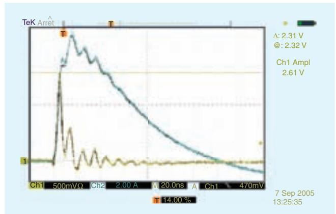
Fig. 12. Reference measurement, outside the box. Chan. 1: Field radiated with current injected on an external,vertical rod, simulating the lightning channel. Chan. 2: injected current.
