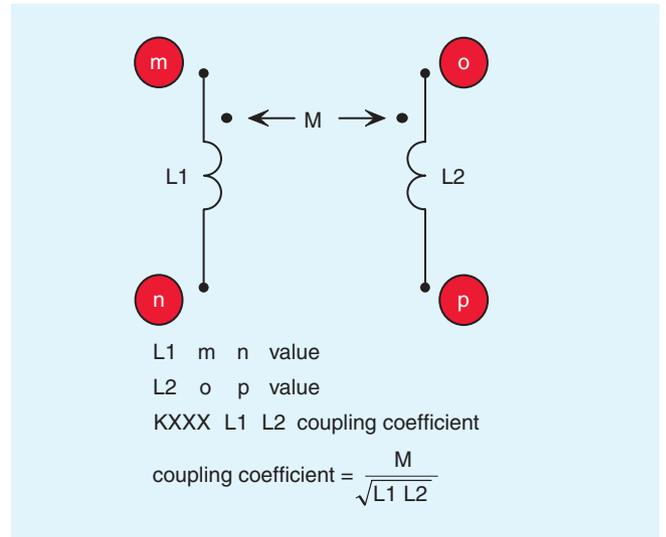
Fig. 4. Coding convention for mutual inductance between two coupled inductors.
