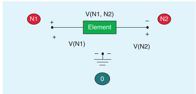
Fig. 1. Node voltage and element voltage notation in the SPICE (PSPICE) circuit analysis program.
