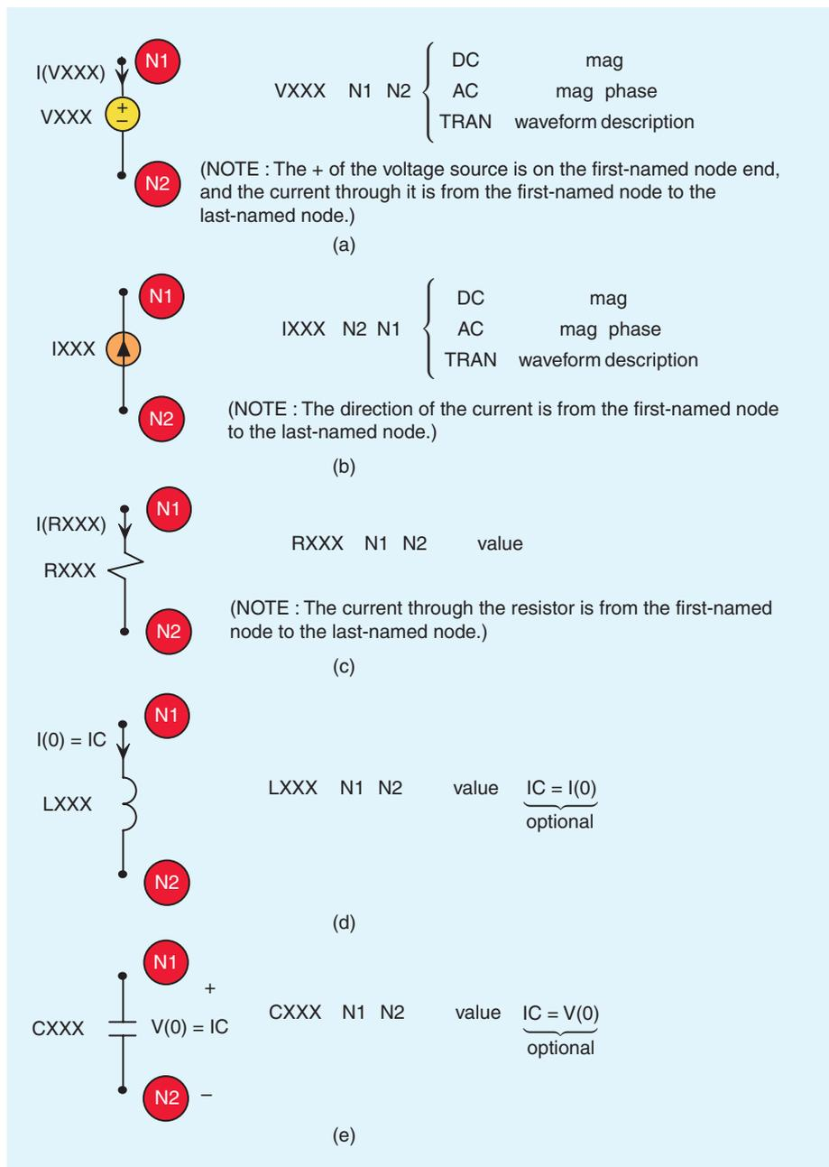
Fig. 2. Coding convention for (a) the independent voltage source, (b) the independent current source, (c) the resistor, (d) the inductor, and (e) the capacitor.
