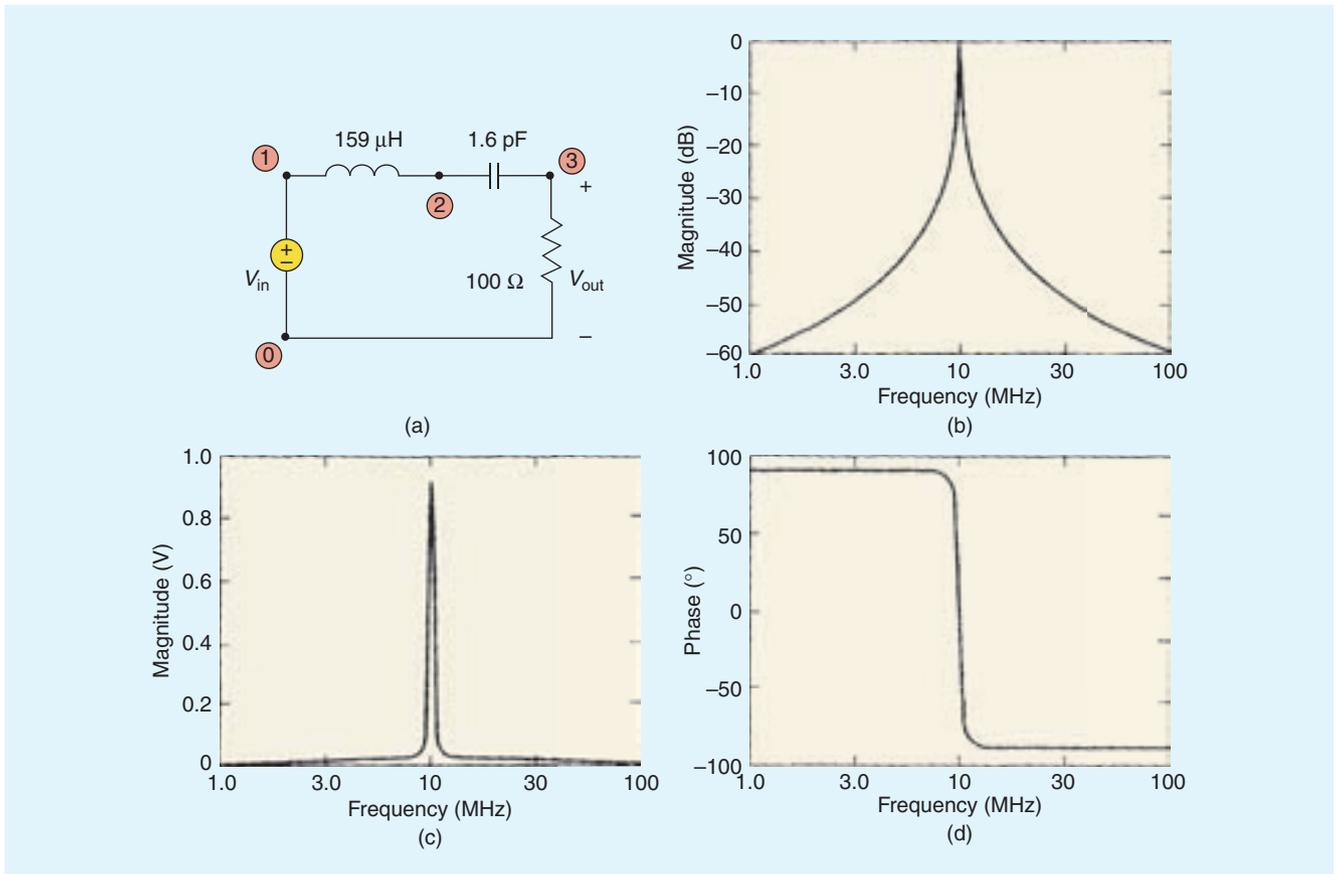
Fig. 8. Example 2, an example of a AC analysis.
