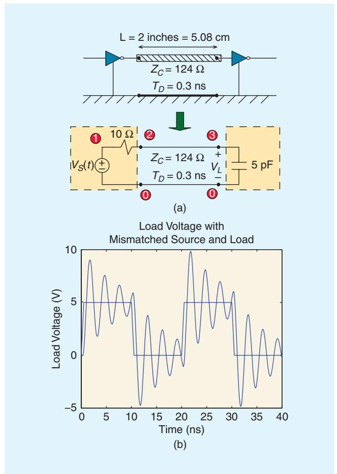
Fig. 10. Example 4, an example of a Signal Integrity analysis.
