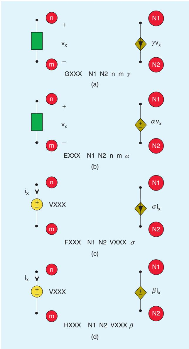
Fig. 3. Coding convention for (a) the voltage-controlled current source, (b) the voltage-controlled voltage source, (c) the current-controlled current source, (d) the current-controlled voltage source.
