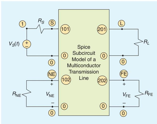
Fig. 11. Connection of a SPICE subcircuit model of a multiconductor transmission line (MTL) to its terminations.
