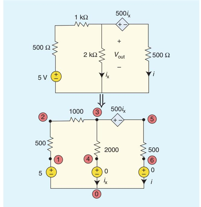
Fig. 7. Example 1, an example of a DC analysis.
