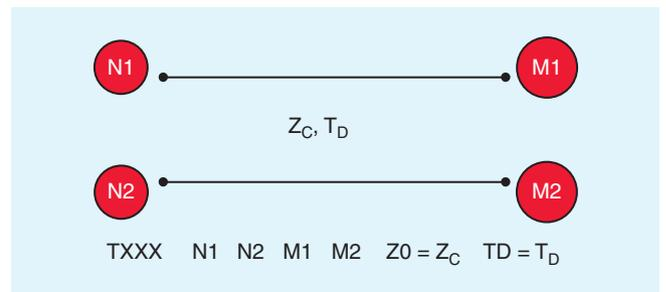
Fig. 5. Coding convention for the two-conductor, lossless transmission line.
