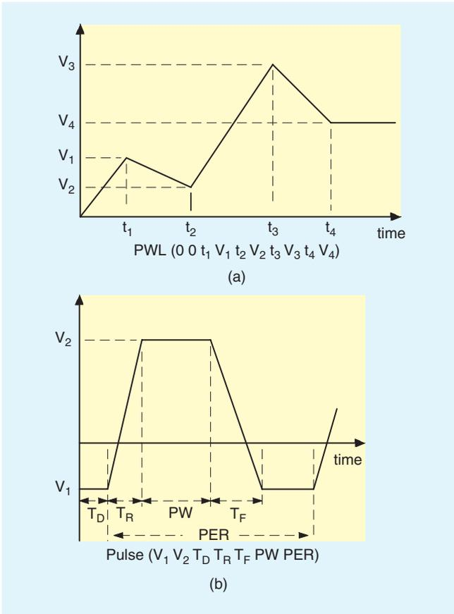
Fig. 6. Coding convention for the important source waveforms: (a) the piecewise-linear waveform and (b) the pulse source waveform (periodic).
