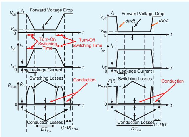
Fig. 6. Voltage, current and power waveforms of a switch at two different switching times.
