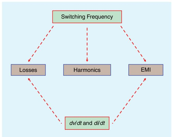
Fig. 8. A relationship between Losses, EMI and Harmonics.
