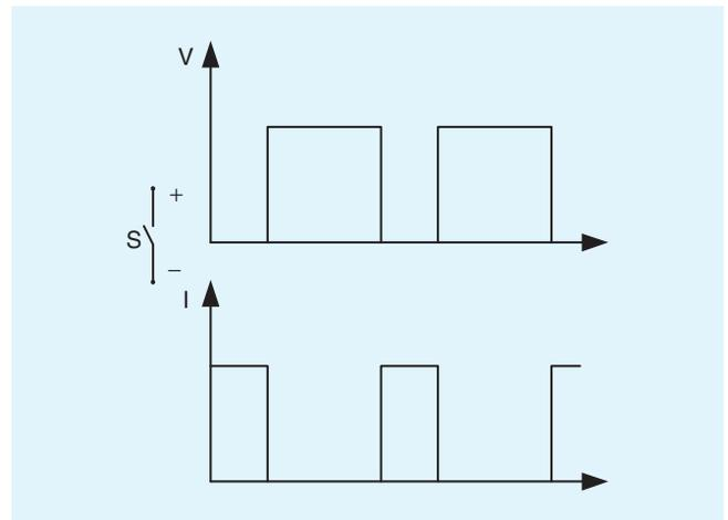
Fig. 3. Voltage and current waveforms in an ideal switch.
