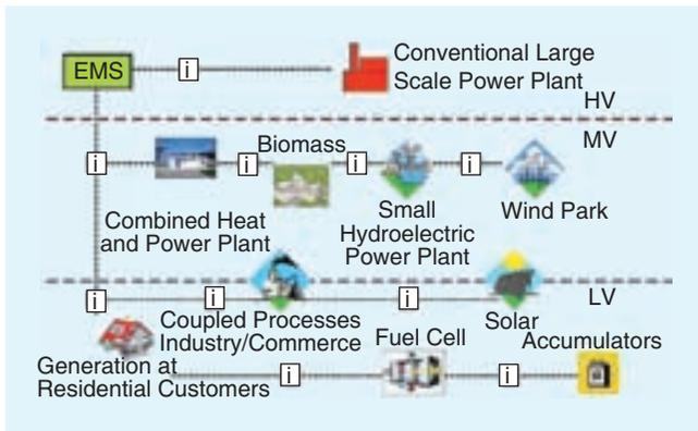
Fig. 6. Example of distributed power generation.
