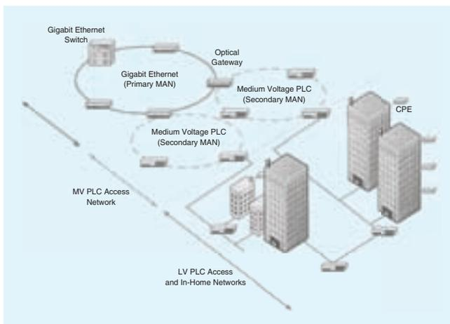
Fig. 3. Example of a typical PLT topology.
