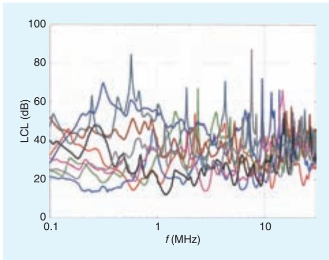
Fig. 2. LCL values measured at various power network sockets by the University of Dortmund.
