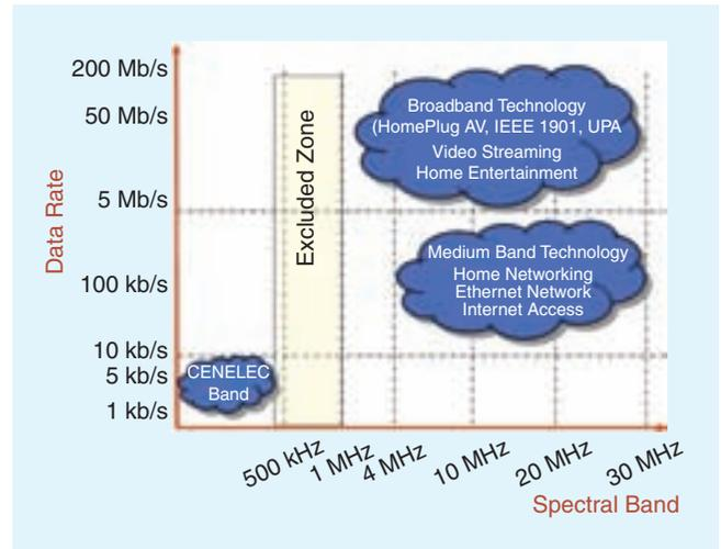
Fig. 1. Power line communication applications.
