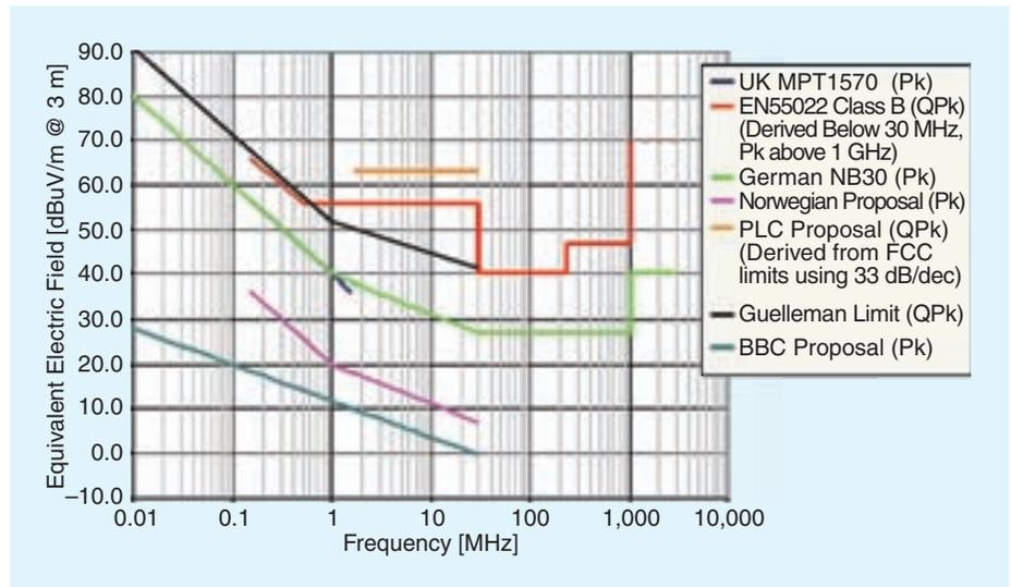
Fig. 4. Electric field limits proposed by different regulatory bodies for PLC emission.
