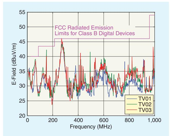
Fig. 2. Far-field radiation measurement on three TVs.
