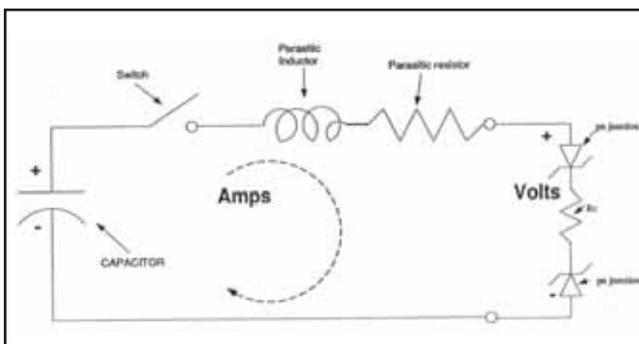
Fig. 8. Typical Firing Circuit.
