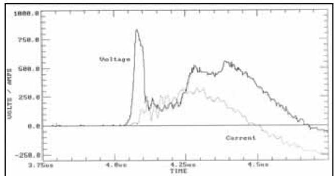
Fig. 9. Current and voltage of a typical firing.
