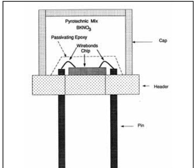
Fig. 3. A pictorial representation of a packaged device.
