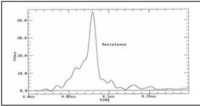
Fig. 10. Ratio of voltage to current for typical firing.
