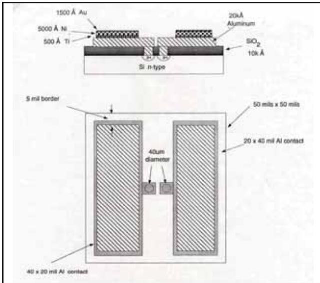
Fig. 2. Pictorial representation of the device.
