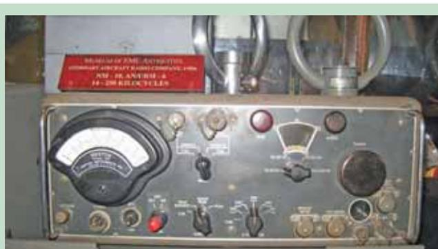
*One of the instruments used in the Greek Island Survey: The Stoddart NM-10, a 14 kHz to 250 kHz receiver. Photo courtesy of Ken Javor and the Museum of EMC Antiquities.*
