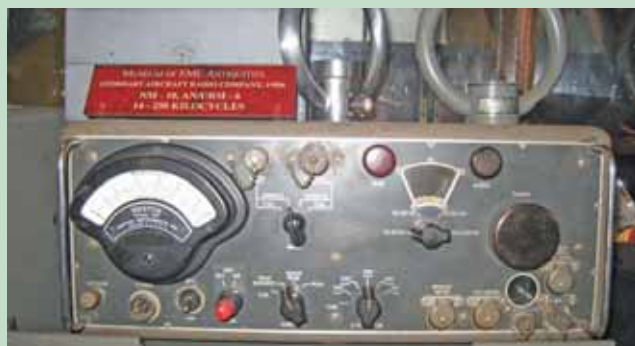
One of the instruments used in the Greek Island Survey: The Stoddart NM-10, a 14 kHz to 250 kHz receiver. Photo courtesy of Ken Javor and the Museum of EMC Antiquities.
